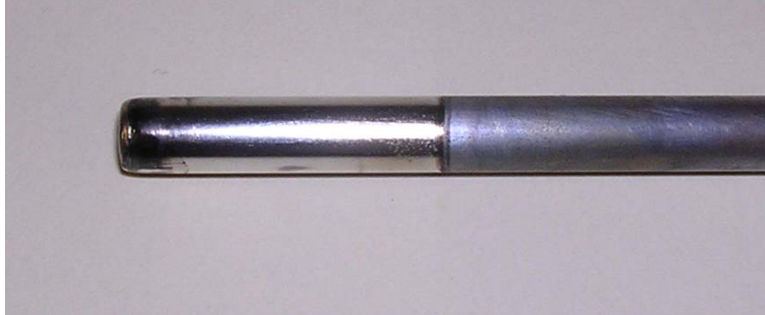
a bright deposit of aluminium on a rod of mild steel.
