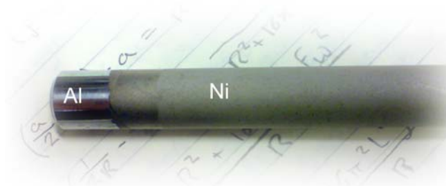
10 mm (dia.) Al rod coated with electroless Cu and then adherent electrolytic Ni (10 \mu\text{m} )
