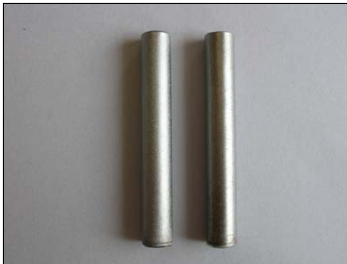
Sample with Hard chromium deposit: (thickness: 25-30 \mu\text{m} )
