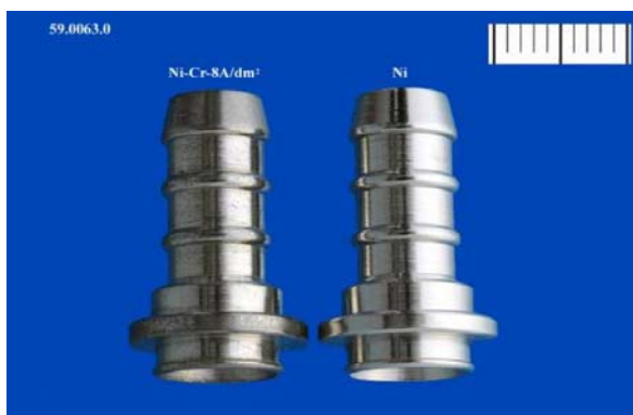
Decorative Chromium on steel from ionic liquids on various samples (INASMET)
