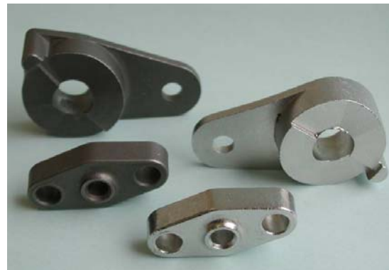
Pieces polished using ionic liquids
