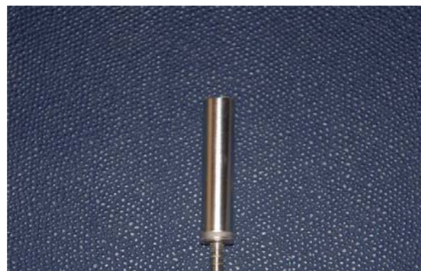
Zn-Sn (10% Zn content) on mild steel
