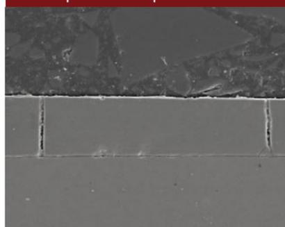
Cross section of a deposit on steel (thickness: 30 µm)
