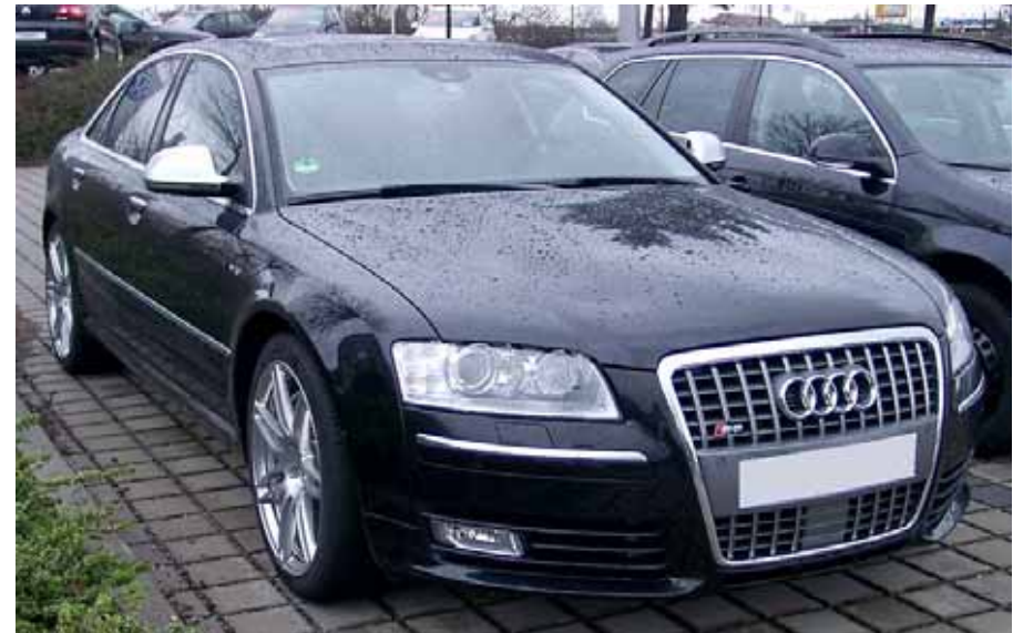
Audi A8 (Full Aluminum Car Body)
